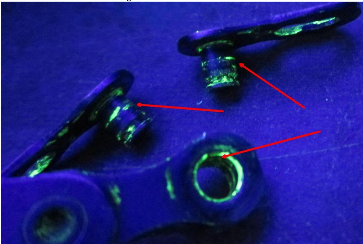
After the ride, the pins of the PowerLock master link were coated in a film of **Bike Milk**. The film is most concentrated in the middle of the pin where the cylindrical spigots of the inner plates join and leave a small gap. Considering this inspection was made after a 2h ride in dry conditions, there is a surprisingly large “reservoir” of **Bike Milk** film located in between the roller and the spigots.
