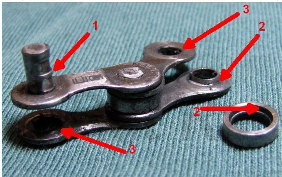
It is well understood that the three areas where most chain wear occurs are **1)** between the outside of pins and the inside of the spigots, **2)** between the outside of the spigots and the rollers, **3)** between the outer plates and the inner plates. These are the areas which require most effective lubrication.
