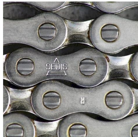
In the US patent Dupoyet used the following descriptions for the most important parts of his invention: 1<sup>c</sup> inner plates; 1<sup>d</sup> outer plates; 8 roller; 10 spacer members (solid or hollow pins); 11 cylindrical spigots. The pins are riveted through the outer plates at point 12<sup>b</sup> and do not rotate at that point. Not much has changed in the basic design although some chains are now narrower to match the increased number of cogs on the cassette.
