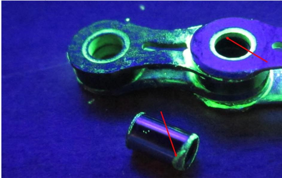
Investigating a master link does not give a perfect indication of what happens inside the standard pins/spigots of a chain as it is a much looser linkage. However, it does provide a useful indication of **Bike Milk** penetration to the innermost chain cavities. The benefit to using a master link is that it can be more easily removed from the outer plate without being “wiped” by the outer plate.
