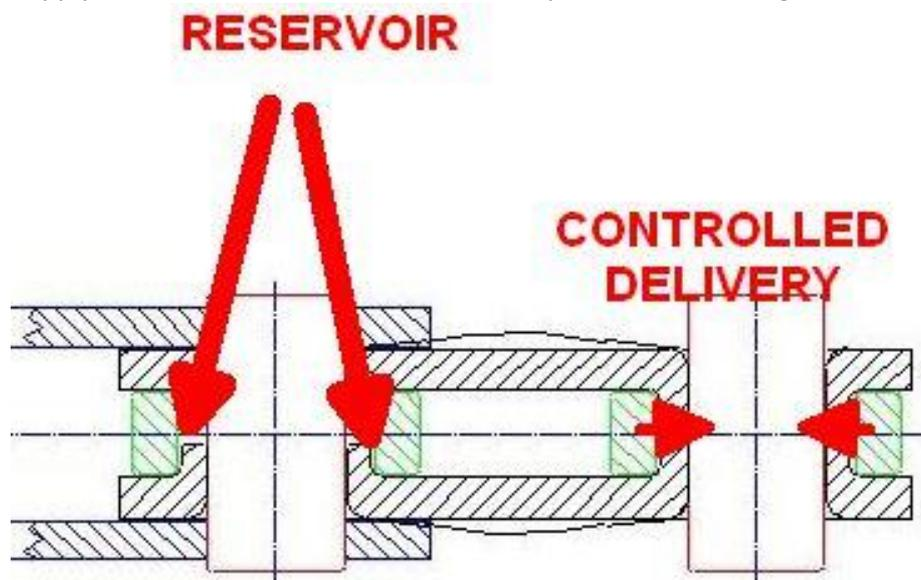
After a MTB ride in dry dusty conditions, and despite there being negligible lubricant coating on the surface of the chain or drivetrain, the inner surfaces of the chain remain well lubricated and the drivetrain performance is maintained.
